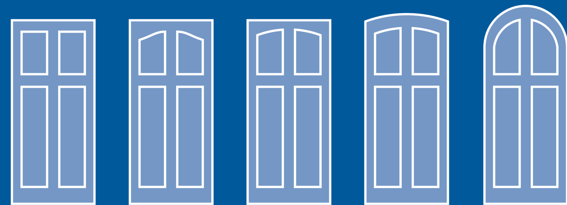
SQUARE PANEL CATHEDRAL ARCH ROMAN ARCH ARCH TOP RADIUS TOP DOOR SHAPES
